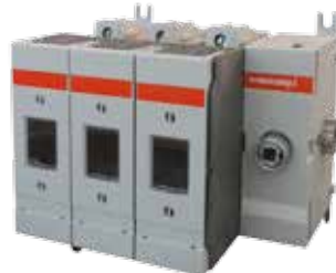
M60J30 60A, J fused, with 3 poles on left side of handle
